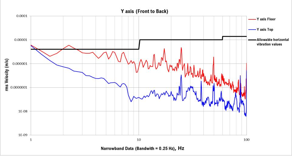
The subway trains caused floor vibration at 2.25 Hz in y axis, which exceeded the horizontal allowable vibration values. Our active vibration isolation system reduced the floor vibration from VC-D to VC-G, meeting the electron microscope's vibration specification.
