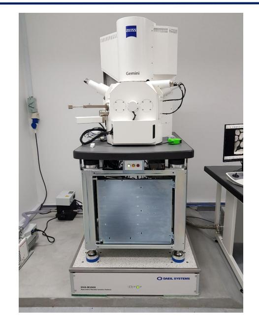
The installation site is located near a subway station, caused the low frequency floor vibration in vertical and horizontal axis that the measured floor vibration levels did not meet the ZEISS Gemini SEM vibration specification. DAEIL SYSTEMS's active vibration isolation system reduced the floor vibrations in Z, X and Y axis, succeeded in meeting the vibration specification.
