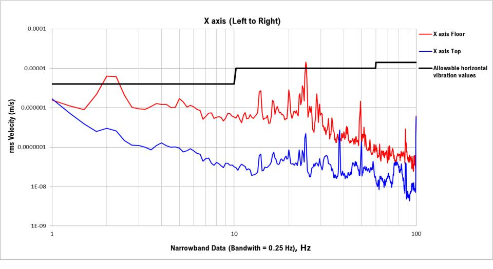
The subway trains caused floor vibration at 2 Hz and 25 Hz in x axis, which exceeded the horizontal allowable vibration values. Our active vibration isolation system reduced the floor vibration from VC-D to VC-G, meeting the electron microscope's vibration specification.
