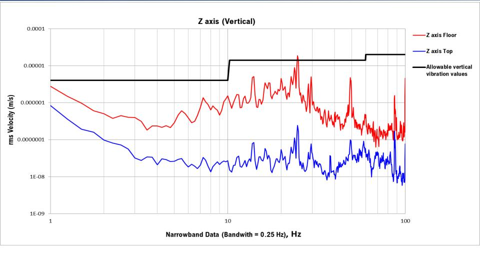
The subway trains caused a significant amount of vibration in Z axis at 25 Hz, at which point the floor vibration exceeded the allowable vertical vibration values for ZEISS Gemini SEM. Our active vibration isolation system reduced the 25 Hz floor vibration, meeting the vertical vibration specification.
