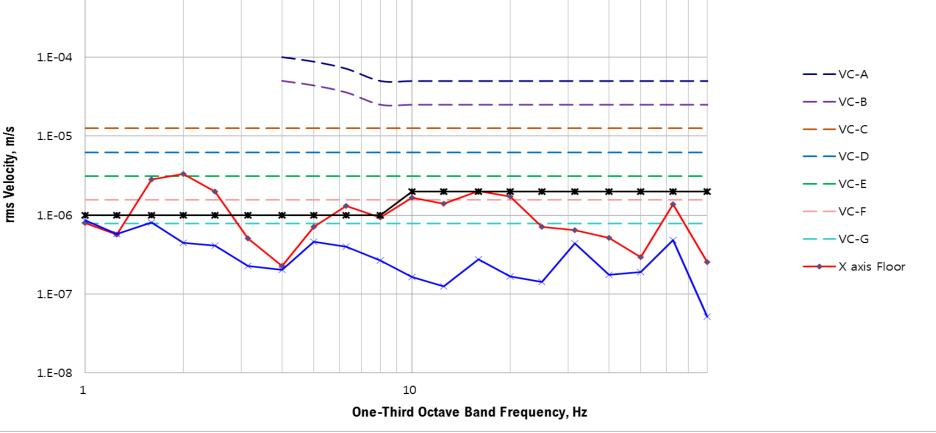
The measured floor vibration in X axis below 10 Hz exceeded the allowable floor vibration. DAEIL SYSTEMS's active vibration isolation system reduced the floor vibration from VC-E to VC-G in 1 - 80 Hz, meeting the floor vibration specification.
