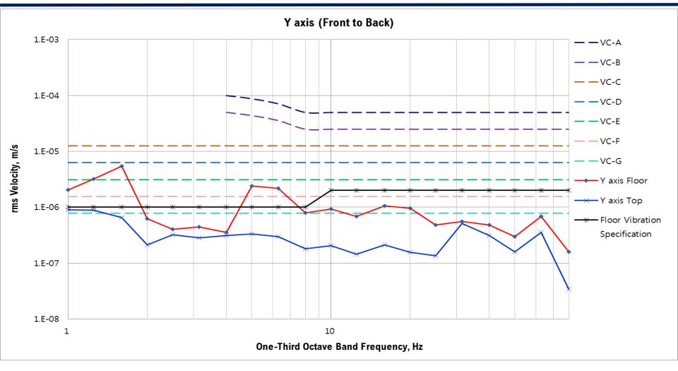
The low frequency floor vibration at 1.6 Hz, 5 Hz, 6.3 Hz exceed the allowable floor vibration values. DAEIL SYSTEMS's active vibration isolation system reduced these vibrations, achieved to meet the floor vibration specification.
