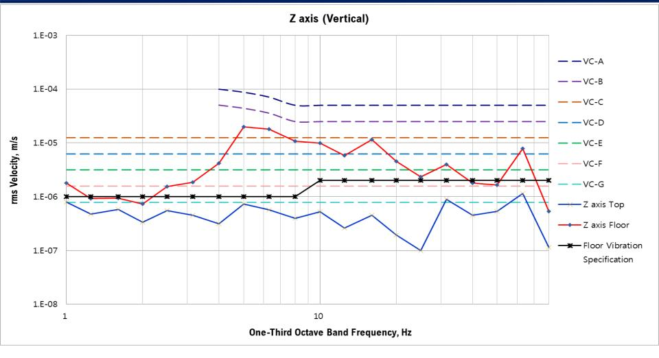
The measured vertical floor vibration exceeded the allowable floor vibration values from 1 to 80 Hz. After the installation of DAEIL SYSTEMS's active vibration isolation system, the floor vibrations were reduced to meet the floor vibration specification.
